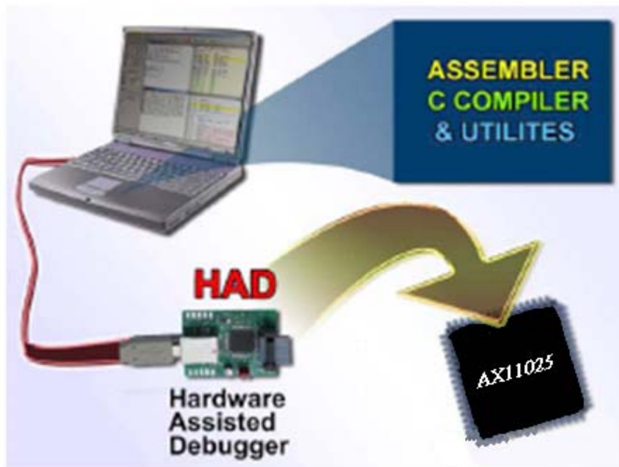
Figure 5: Typical Debugger and Hardware Assisted Debugger (HAD2) System Diagram
