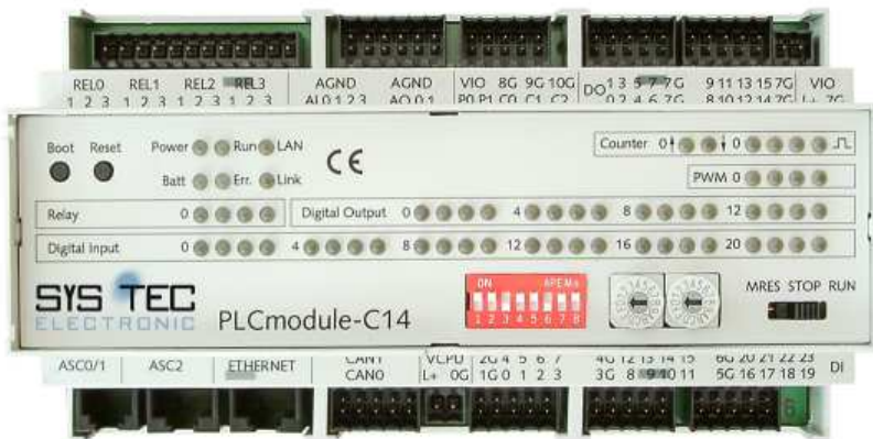
Figure 2: Top-view of the PLCmodule-C14 (top side)
