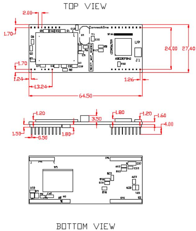
Figure 5-1: Mechanical Dimensions
